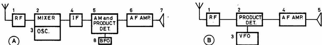
Fig. 1A shows the arrangement of the standard superhet while Fig. 1B illustrates the reduced number of stages required for a direct conversion receiver.
