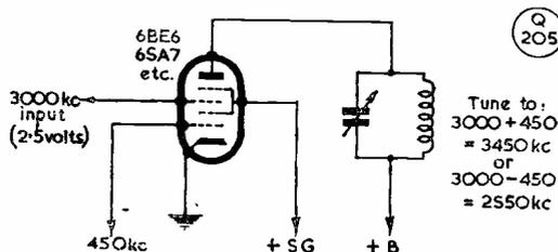
Fig. 2. Pentagrid mixer suitable for SSB frequency conversion. A 450 kc SSB signal is fed to grid 1, and the conversion frequency RF signal to grid 3. The plate circuit is tuned to the sum or difference of the two input frequencies; in this example, the output could be either 3,450 or 2,550 kc.
