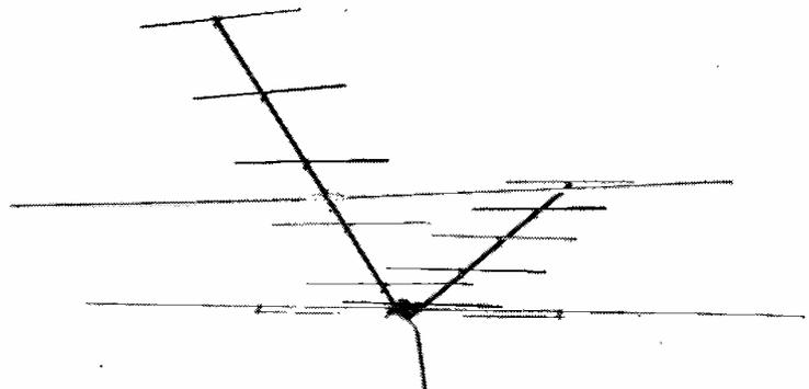
The Labgear type C.30 aerial assembly is a special three-channel model designed to cater for one Band I and one Band III transmission originating from one direction, and an additional Band III service from a completely different direction.
