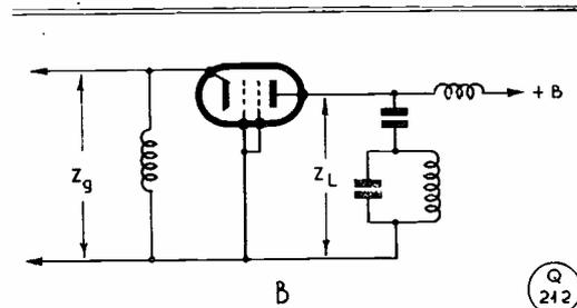
Fig. 9 (A). Input and output impedances of a grounded grid linear amplifier appear in shunt to the driver. Any change in one has a reaction on the other; this can demand high drive. Fig. 9 (B) shows the circuit for a grounded-grid, grounded-screen amplifier. Many pentodes or tetrodes may be used in this configuration with good results; in the case of a pentode with separate suppressor, this should be tied to the other two grids.
