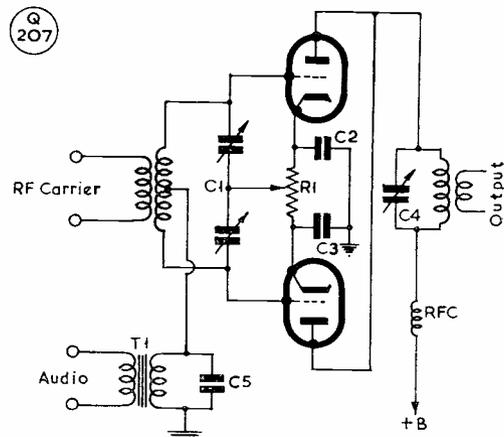
Fig. 4. The push-push balanced modulator with grid and plate circuits resonated for the RF carrier frequency. Both the RF excitation and the audio are in push-pull, with the output in parallel. C1, C4 are tuned to the carrier frequency, and R1 set for minimum carrier output. As in the case of Fig. 3, a DSB signal appears in the tank circuit.
