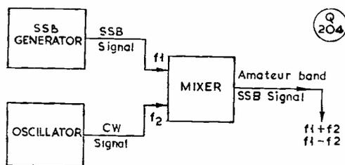
Fig. 1. A mixer stage fed by two signal generating stages. The SSB signal,  $F_1$ , and the RF carrier,  $F_2$ , are heterodyned to produce two new beats, the sum and difference of  $F_1$  with  $F_2$ . Careful selection of the two signal frequencies is necessary to eliminate the possibility of spurious beats appearing with the wanted signal.
