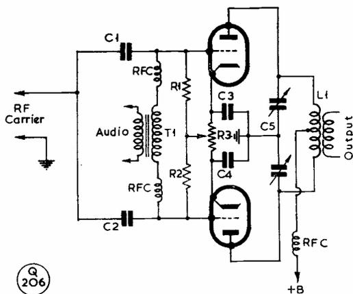
Fig. 3. Typical push-pull balanced modulator. The RF drive is introduced in parallel in both valves and the audio modulating frequency in push-pull. The carrier is suppressed in the push-pull tuned output circuit, with only the two sideband frequencies remaining—thus, a double-sideband suppressed-carrier signal. In practice, C5 is tuned to the RF input signal and the cathode bias potentiometer R3 adjusted for maximum carrier suppression.
