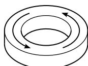
*Apply a strong clockwise external field. This switches the core's magnetism, and the core now has clockwise magnetism:*
