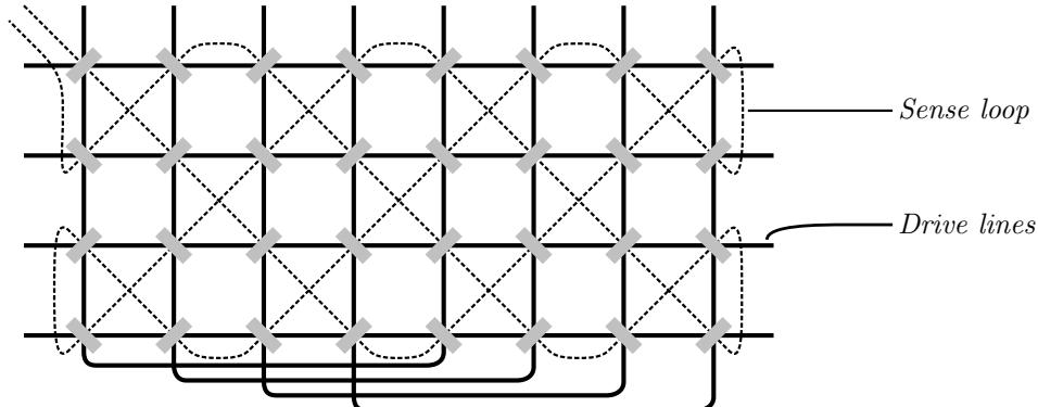
The array of cores can be thought of as two halves, with each core in the left half having an anti-coincident partner in the right half sharing the same pair of drive lines.
