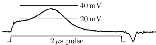
*However, if the applied field is in the same direction as the core's existing magnetisation, no switching takes places, and we observe a negligible voltage:*
