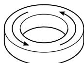
*Apply a weak clockwise external field. This reduces the strength of the anti-clockwise magnetism in the core:*
