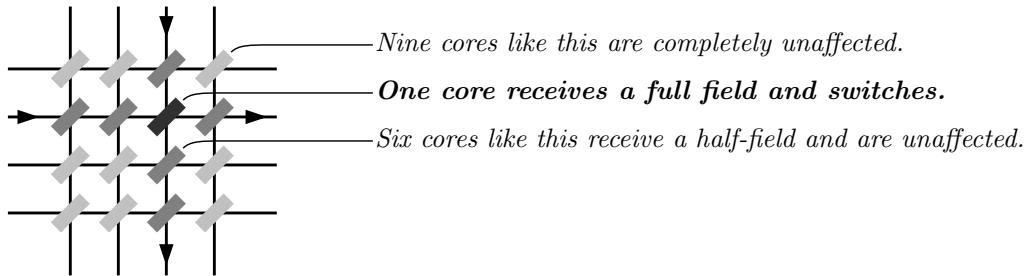
We only need  $O(\sqrt{N})$  drive lines for an array of  $N$  cores.
