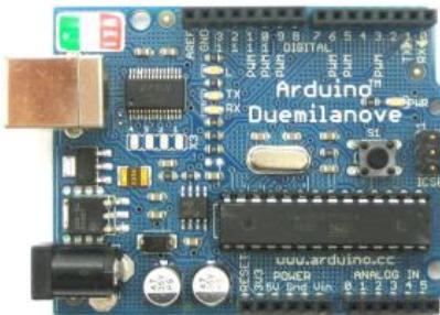
**The Arduino is a popular, easy-to-use, open design microprocessor board with IO capabilities.**
