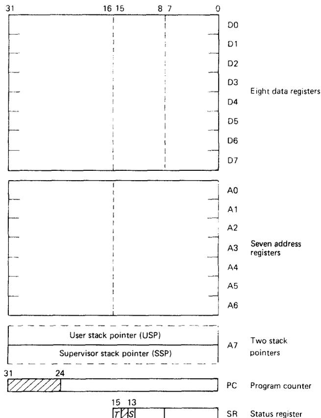
Figure 1. MC68000 programming model
