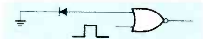
FIG. 7—A DIODE IS USED to imitate a "high" input for an ECL gate.
