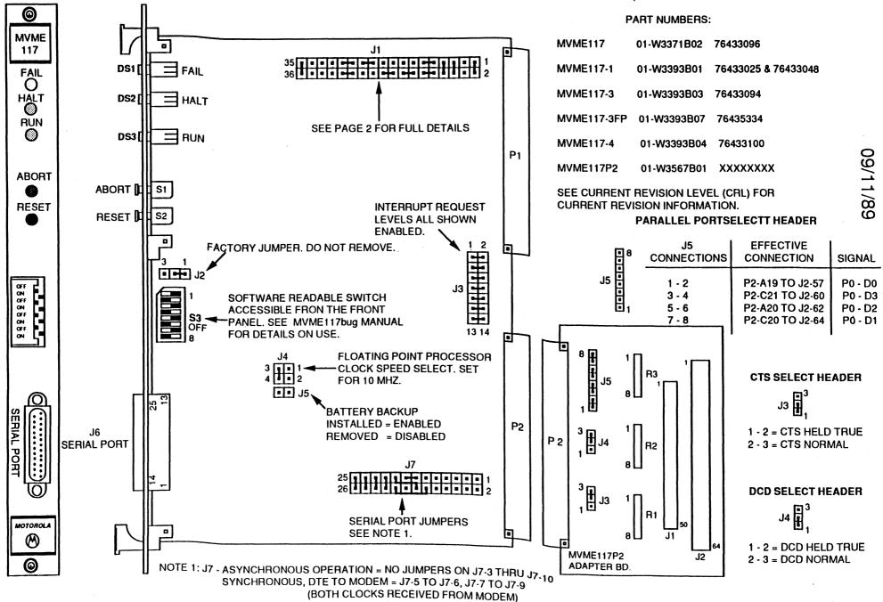
SYNCHRONOUS, DCE TO TERMINAL = J7-3 TO J7-4, J7-5 TO J7-7, J7-8 TO J7-10
