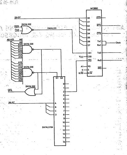
Figure 1. MC6800 to MC6850 Interconnections
